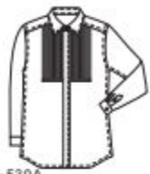
S-530A Accordion pleats front with pleated patch(13 0.7cm width pleat each side)
